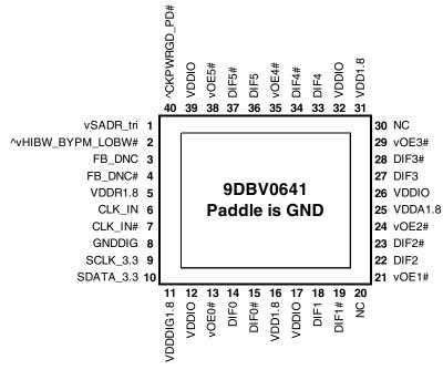
**40-pin VFQFPN** ^ prefix indicates internal Pull-Up Resistor v prefix indicates Internal Pull-Dow n Resistor 5mm x 5mm 0.4mm pin pitch
