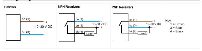
Quick disconnect wiring diagrams are functionally identical.
